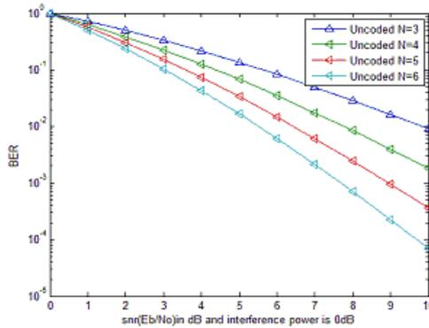
Fig.2 ber for uncoded oc system
