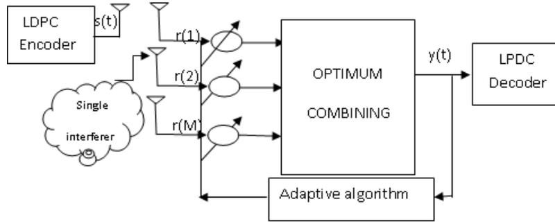
Fig.1 system model of ldpc-oc with single interferer
